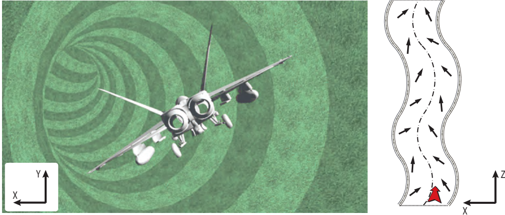
Fig. 4. Left figure presents the flight simulator, in which the movements of the plane is coupled to the rotations of the 3RPS-R end-effector. Right figure depicts cross section of tunnel on which virtual walls and velocity field are depicted schematically.
